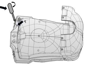
Wrap cable around and over the base & foam. Close chest making sure cable is sandwiched between skin and foam. Note: Skin may not fully latch on side where cable is routed.
