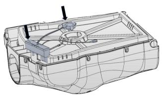
Carefully insert piston plug and make sure plug is fully sealed.
